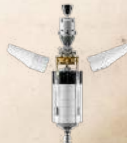
After docking, the CSM pulls the LM away from the launch vehicle's upper stage
